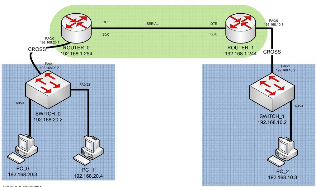
ROUTER\_0: CISCO 2611 ROUTER\_1: CISCO 2610 SWITCH: CISCO CATALYST 2924XL DATED: 10<sup>TH</sup> OF MARCH 2010
